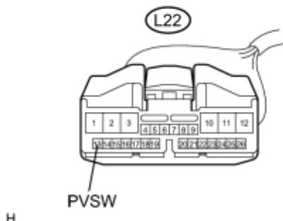
(a) Disconnect the solar ventilation ECU connector.
