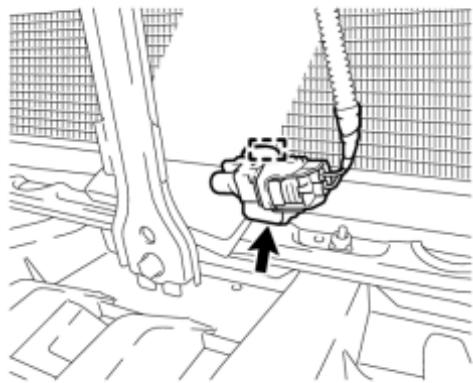
(a) Engage the clamp to install the ambient temperature sensor.
