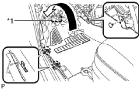
(c) Engage the fastener to install the floor carpet to the original position as shown in the illustration.
