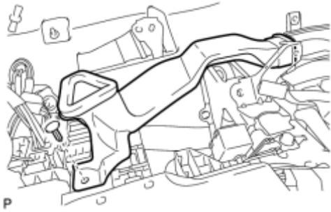
(a) Remove the clip and No. 3 side defroster nozzle duct.
