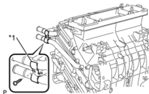
(a) Remove the screw and clamp.
