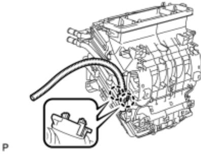
(a) Disengage the 2 claws and remove the air conditioning duct sub-assembly.
