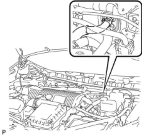
(a) Using pliers, grip the claws of the clip and slide the clip to connect the inlet heater water hose.
