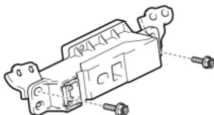
(a) Install the plasmacluster with the 2 screws to the 2 brackets.
