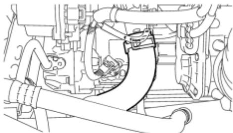
(a) Using pliers, grip the claws of the clip and slide the clip to remove the No. 2 radiator hose.
