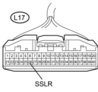
(b) Disconnect the A/C amplifier connector.
