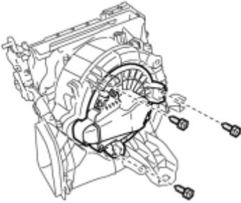
(a) Remove the 3 screws and front blower motor sub-assembly.
