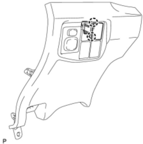
(a) Disengage the 2 claws and remove the solar ventilation switch.
