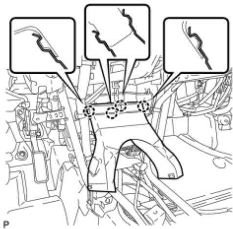
(a) Engage the 4 claws to install the rear No. 1 air duct.
