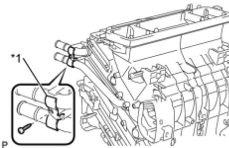
(b) Install the clamp with the screw.
