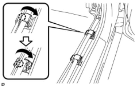
(a) Disengage each claw to open the 2 door scuff plate clamps as shown in the illustration.
