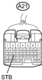
(a) Disconnect the connector from the power management control ECU.
