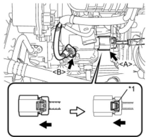
(c) Connect the connector <A> and lock the green-colored lock as shown in the illustration.
