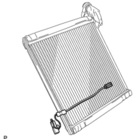
(a) Remove the No. 1 cooler thermistor.
