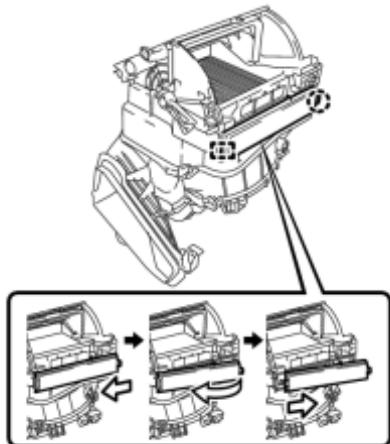
(a) Disengage the claw and guide, and remove the air filter case as shown in the illustration.
