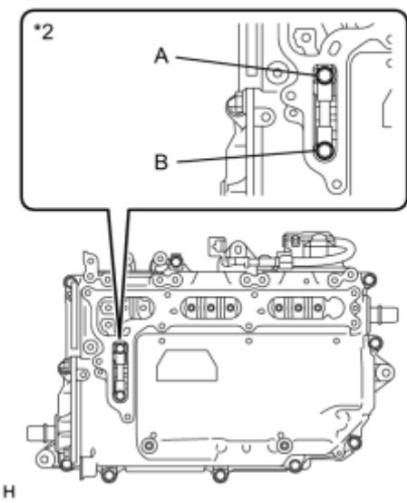
(d) Check that bolts A and B are tightened securely.
