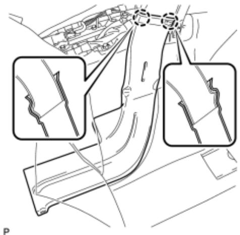
(a) Engage the 2 claws to install the rear No. 3 air duct.
