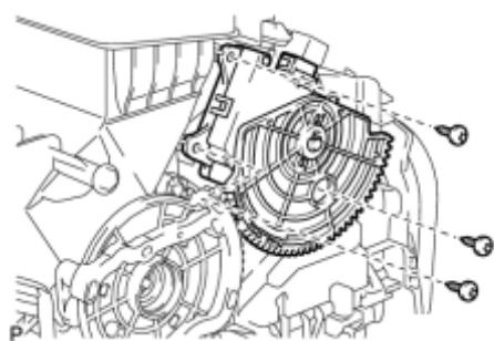
(a) Remove the 3 screws and air outlet control servo motor sub-assembly.
