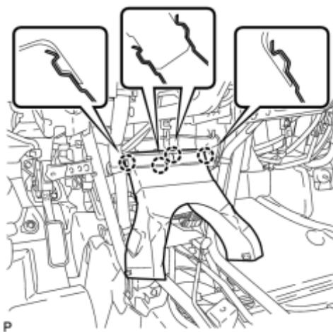
(a) Disengage the 4 claws and remove the rear No. 1 air duct.
