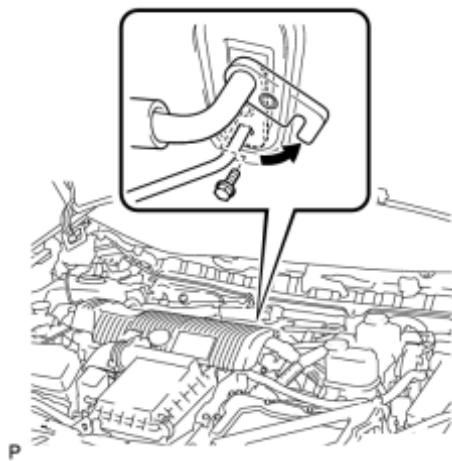
(a) Remove the bolt and slide the hook connector.
