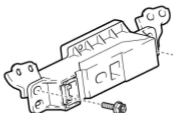
(a) Remove the 2 screws and plasmacluster from the 2 brackets.
