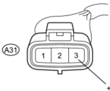
(a) Disconnect the A/C pressure sensor connector.
