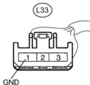
(a) Disconnect the blower motor connector.
