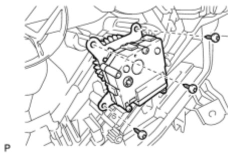
(a) Remove the 3 screws and air mix control servo motor sub-assembly.
