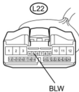
(a) Disconnect the solar ventilation ECU connector.
