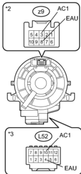
(a) Disconnect the connector from the spiral with sensor cable sub-assembly.
