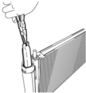
(a) Using pliers, install a new cooler dryer to the modulator.
