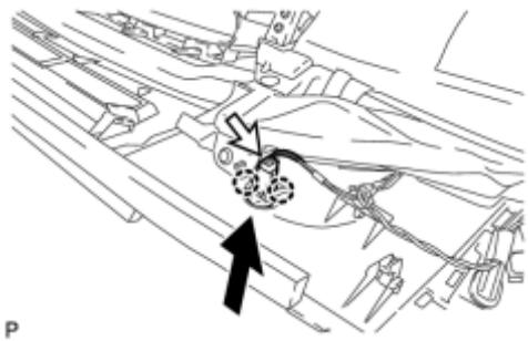
(a) Engage the 2 claws to install the solar sensor as shown in the illustration.
