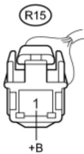
(b) Disconnect the moon roof glass assembly (solar panel) connector.
