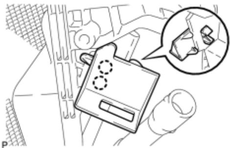
(a) Engage the 2 claws and install the console mounting bracket RH.
