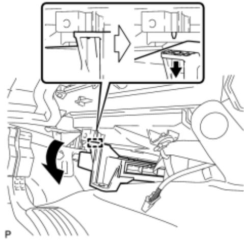
(b) Disengage the guide as shown in the illustration.
