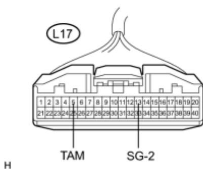
(a) Disconnect the A/C amplifier connector.
