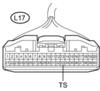
(b) Disconnect the A/C amplifier connector.
