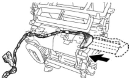
(a) Install the quick heater assembly as shown in the illustration.
