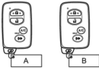
(2) Operate the remote A/C switch on key (electrical transmitter) A and check that the remote air conditioning system can be operated.
