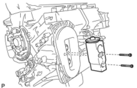
(a) Using a 4 mm hexagon wrench, install the cooler expansion valve with the 2 hexagon bolts.
