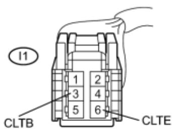
(a) Disconnect the solar sensor (automatic light control sensor) connector.
