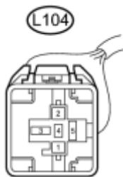
(a) Disconnect the solar ventilation relay connector.
