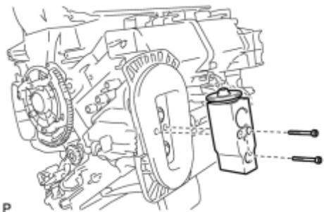
(a) Using a 4 mm hexagon wrench, remove the 2 hexagon bolts and cooler expansion valve.
