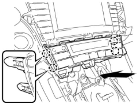
(b) Engage the 4 claws to install the air conditioning control assembly.
