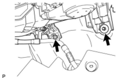
(a) Install the air conditioning unit assembly with the bolt and nut.
