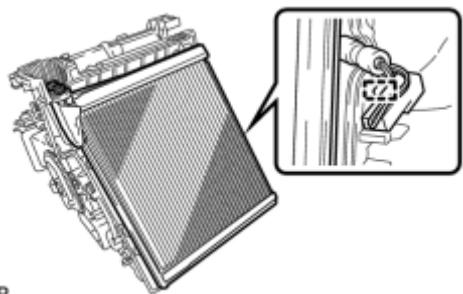
(d) Disengage the clamp and remove the cooler evaporator sub-assembly with the No. 1 cooler thermistor.
