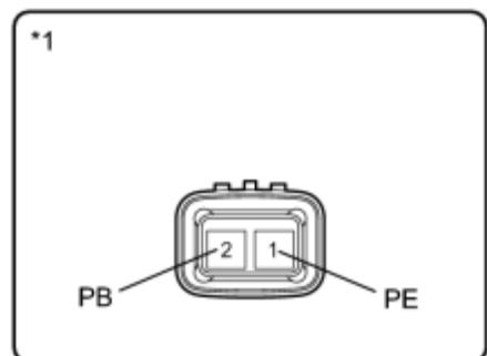
(a) Disconnect the compressor with motor assembly connector.
