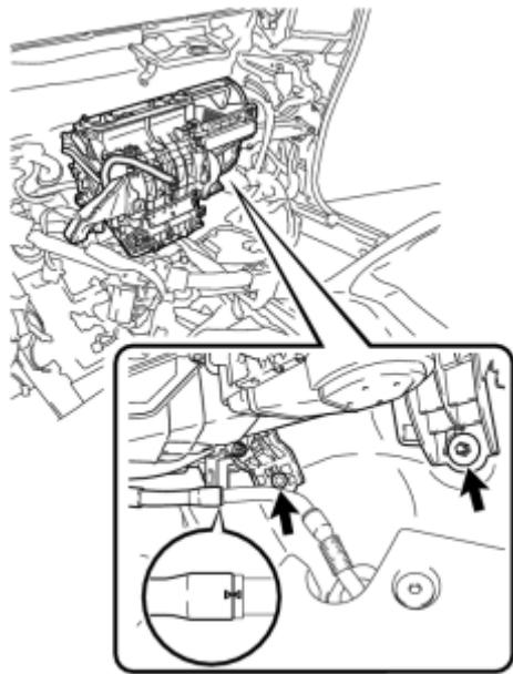
(a) Temporarily tighten the air conditioning unit assembly with the bolt and nut.
