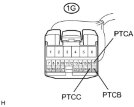
(b) Disconnect the engine room relay block and junction block (integration relay) connector.
