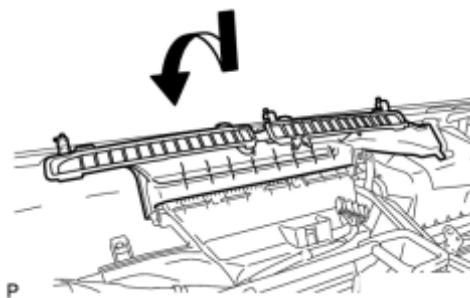
(a) Install the defroster nozzle assembly as shown in the illustration.
