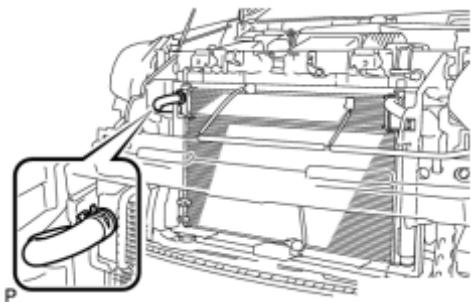
(a) Using pliers, grip the claws of the clip and slide the clip to connect the No. 5 inverter cooling hose.
