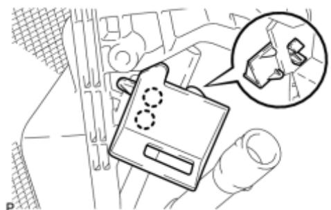
(a) Disengage the 2 claws and remove the console mounting bracket RH.
