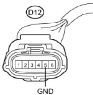
(a) Disconnect the connector from the compressor with motor assembly.
