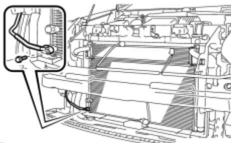
(a) Remove the bolt and disconnect the air conditioning tube and accessory assembly.
