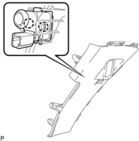
(a) Engage the 2 claws to install the room temperature sensor to the No. 1 switch hole base.
