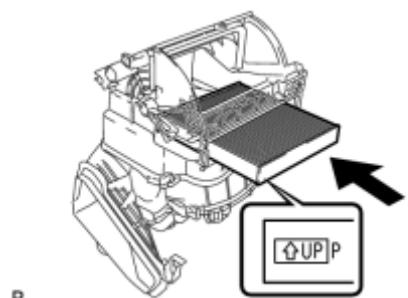
(a) Install the clean air filter as shown in the illustration.
