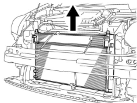
(a) Remove the cooler condenser assembly with hybrid radiator assembly.
