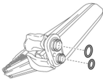
(e) Remove the 2 O-rings from the cooler evaporator sub-assembly.
