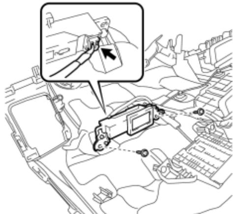
(a) Install the plasmacluster with bracket with the 2 screws.
