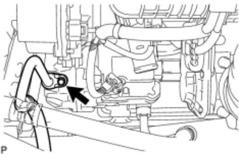
(a) Remove the bolt and disconnect the discharge hose sub-assembly from the electric inverter compressor.
