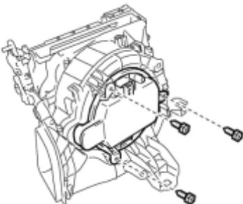
(a) Remove the 3 screws and front blower motor sub-assembly.
