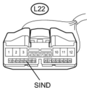
(a) Disconnect the solar ventilation ECU connector.
