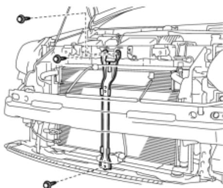
(1) Remove the 3 bolts and millimeter wave radar sensor bracket.
