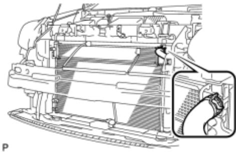
(a) Using pliers, grip the claws of the clip and slide the clip to disconnect the No. 7 inverter cooling hose.
