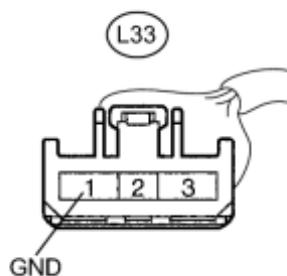
(a) Disconnect the blower motor connector.
