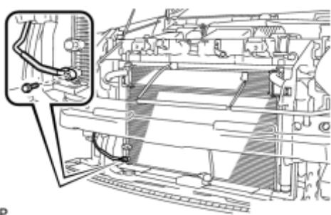
(d) Install the air conditioning tube and accessory assembly on the cooler condenser assembly with the bolt.
