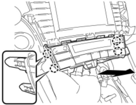
(a) Disengage the 4 claws and remove the air conditioning control assembly as shown in the illustration.
