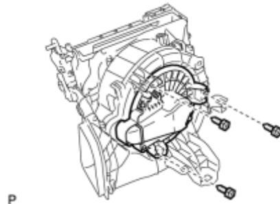
(a) Install the front blower motor sub-assembly with the 3 screws.
