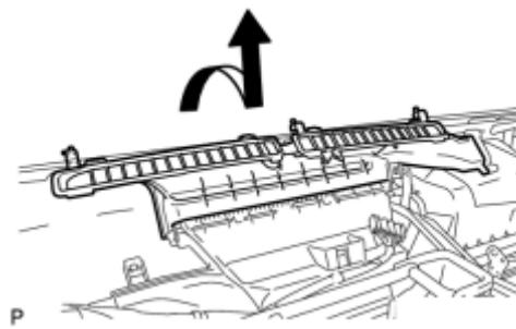
(b) Remove the defroster nozzle assembly as shown in the illustration.
