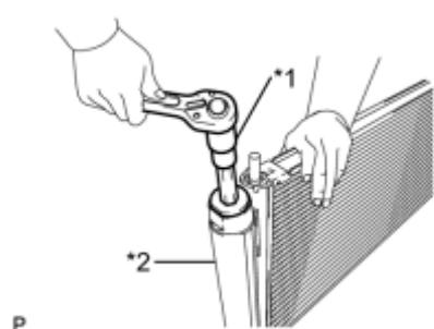
(a) Using a 14 mm straight hexagon wrench, remove the cap from the modulator.
