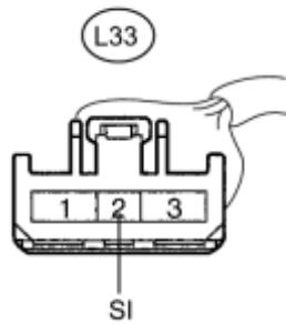
(b) Disconnect the blower motor connector.
