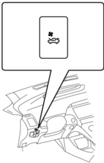
(c) If it is not necessary to operate the solar ventilation system while working on it, turn the solar ventilation switch off.
