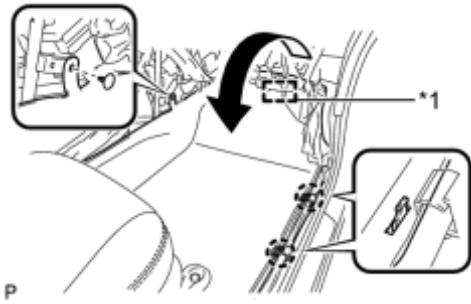
(b) Disengage the clip and fastener.
