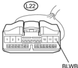
(a) Disconnect the solar ventilation ECU connector.
