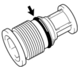
(b) Sufficiently apply compressor oil to a new O-ring and the fitting surfaces of the cap.
