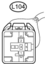
(a) Disconnect the solar ventilation relay connector.
