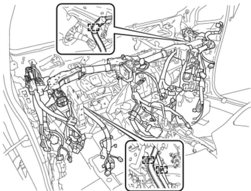
(b) Remove the 9 bolts and instrument panel reinforcement assembly.
