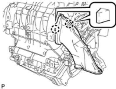
(a) Disengage the 2 claws and remove the No. 1 air duct sub-assembly.
