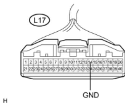
(a) Disconnect the A/C amplifier connector.
