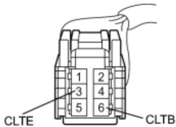
(a) Disconnect the solar sensor connector.
