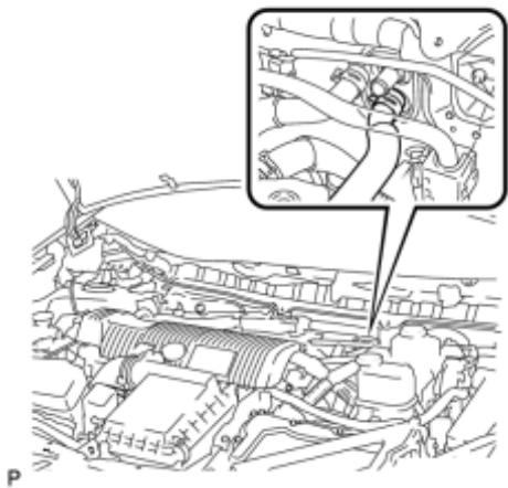
(a) Using pliers, grip the claws of the clip and slide the clip to disconnect the outlet heater water hose.
