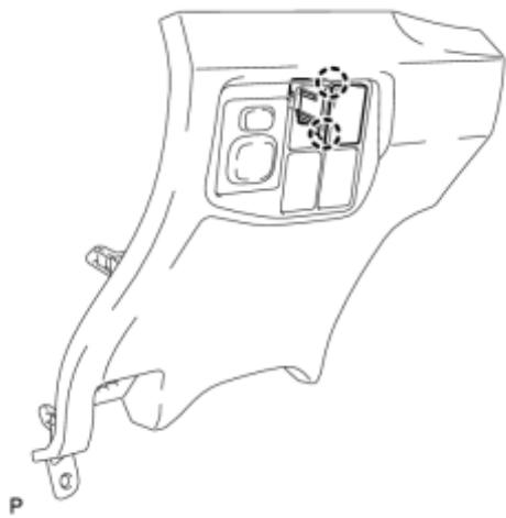
(a) Engage the 2 claws to install the solar ventilation switch.
