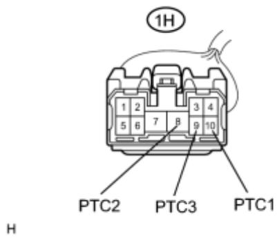
(c) Measure the resistance according to the value(s) in the table below.
