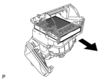
(a) Remove the clean air filter as shown in the illustration.
