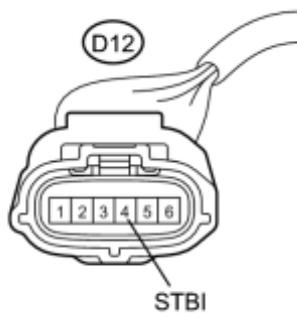
(b) Disconnect the connector from the compressor with motor assembly.
