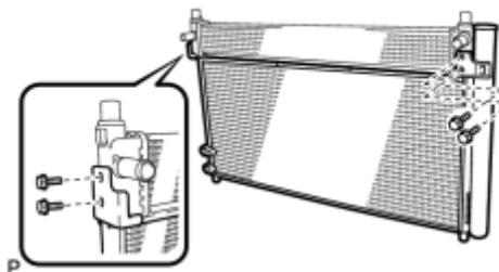
(a) Install the cooler condenser assembly with the 4 bolts to the hybrid radiator assembly.
