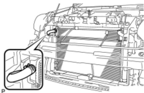
(a) Using pliers, grip the claws of the clip and slide the clip to disconnect the No. 5 inverter cooling hose.
