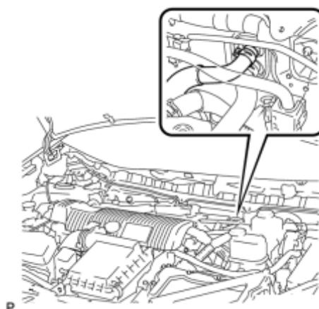
(a) Using pliers, grip the claws of the clip and slide the clip to disconnect the inlet heater water hose.
