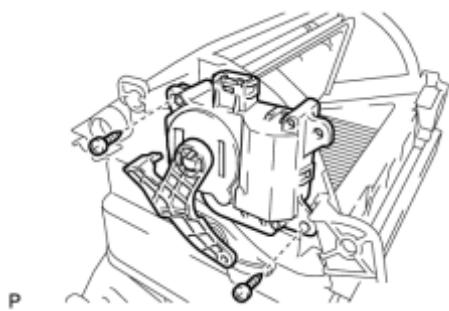
(a) Remove the 2 screws and air inlet control servo motor sub-assembly.
