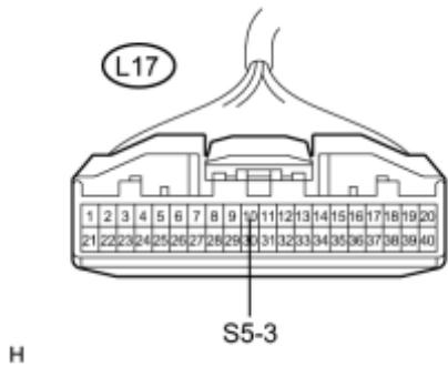
(a) Disconnect the A/C amplifier connector.
