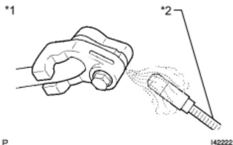
(c) Using a halogen leak detector, inspect for refrigerant leaks from the refrigerant lines.
