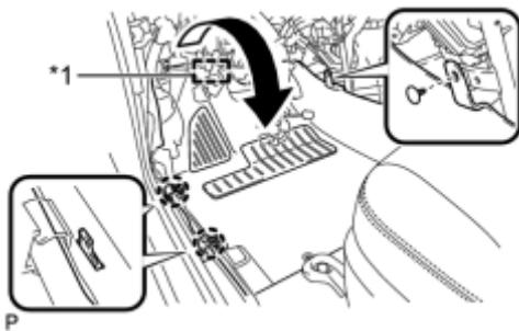
(b) Disengage the clip and fastener.
