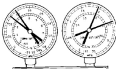
NOTE: These gauge indications occur when the refrigeration system opens and the refrigerant is charged without vacuum purging.
