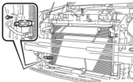
(a) Remove the bolt and disconnect the discharge hose sub-assembly.
