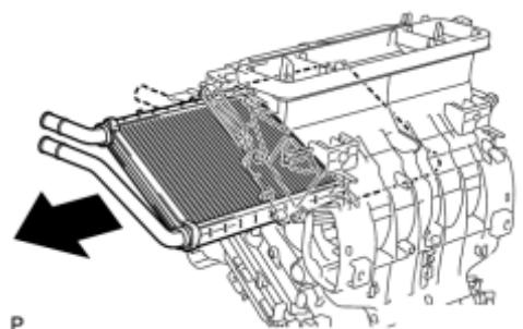
(b) Remove the heater radiator unit sub-assembly as shown in the illustration.
