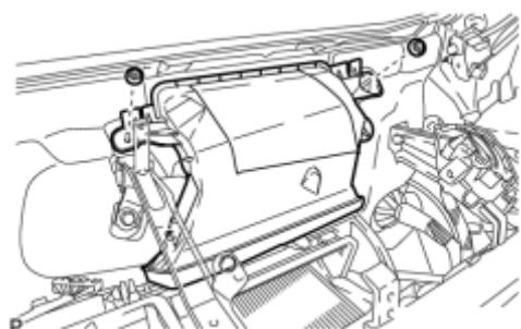
(a) Install the No. 3 air duct sub-assembly with the 2 nuts.
