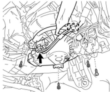
(a) Remove the quick heater connector screw.
